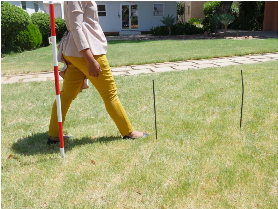
Figure 15: Example of pacing measurement (Primary Data, 2024)
